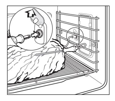
When roasting poultry, the best place to insert the probe is in the thickest part of the bird between the thigh and body.
